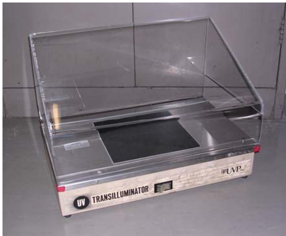
Figure 4 – Photographs showing a suitable form of shield
