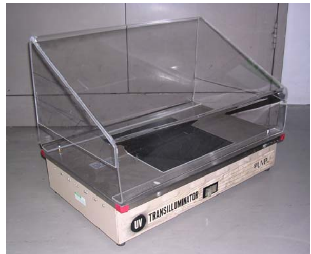
Figure 4 – Photographs showing a suitable form of shield
